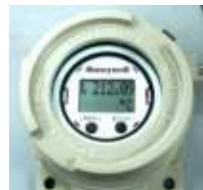
Figure 2 – STT700 Temperature Transmitter with display module
