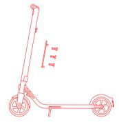
3. Install the external battery on the rail and fix it with the M4 (20mm)Verify that your KickScooter powers on and off. screws (2 pcs) and M3 screw (1 pcs), provided with this product.
