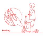
Step on the folding pedal while pushing the handlebar forward
