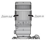
① Using the zoom ring while the lens is wet makes it easier for water to find its way inside the lens. Wipe any water from the lens before using the zoom ring.
